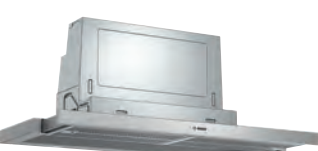
Telescopic Telescopic cooker hoods are installed into a wall unit. To operate them, the flat section is pulled out, enlarging the extraction surface. Selected models have easy installation systems and accessories are available, as well as a lowering frame to make the hood invisible when not in use.
